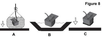
If the hull surface is not smooth, sand it with 30 grit sandpaper until a smooth surface is obtained. Partially fill a thin plastic bag with water, place the transducer inside and close it tightly with a tie wrap. Wet the surface of the hull and press the transducer face against it through the bag.
