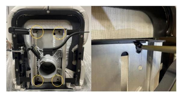
2. Once the slider has been detached, the gas spring should be easy to access for adjustment. It is important to have a protective rubber cover on the gas spring when adjusting. Failure to do so may cause debris to enter the gas spring and prevent it from working properly.
