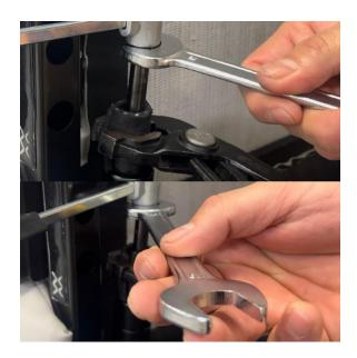
**4.** By turning the cylinder, you can adjust the release lever as necessary until it is tight. Make sure to not overtighten it.
