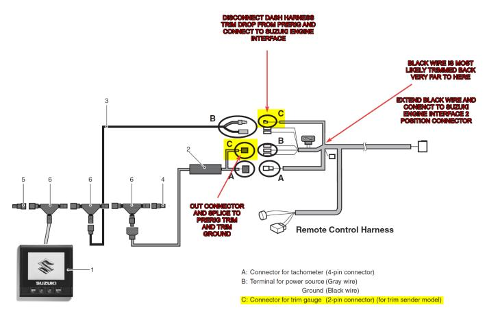
Connect your SDS harness (directional harness, please see tags on each end of harness) to the engine interface and run to the motor. Locate your SDS motor plug and connect the harness to it. Finally, configure your gauge to read Suzuki digital. To do this, please reference the Medallion Analog Gauge Users Guide found on the dealer portal under Manuals/Troubleshooting.
