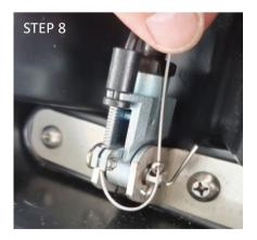
NOTE: The newly installed stainless steel Spring will keep the Gas Spring Release Head trigger Cradle pushed away from the cable Gland
