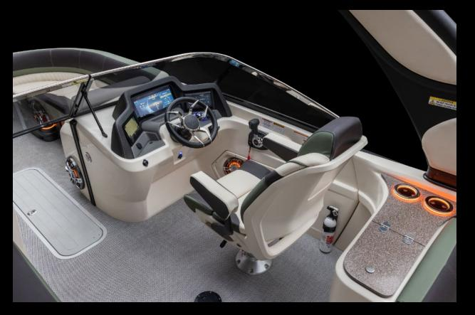
Medallion Viper III touchscreen with automatic & manual wake controls and adjustable electric actuators to press Waveshaper fins. There are multiple adjustment angles to find the perfect wave for each rider. Once the perfect wave and speed is achieved based on rider preference, that can be saved as a preset for future rides tailored to the individual rider.
