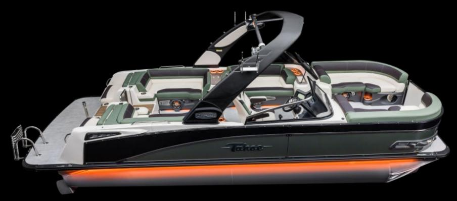
LOA with integrated swim platform: 24' 11" Width: 8' 6" Weight with engine: 5120lbs Engine & Drive weight: 1100lbs
