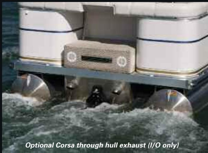
Optional Corsas through hull exhaust (I/O only)
