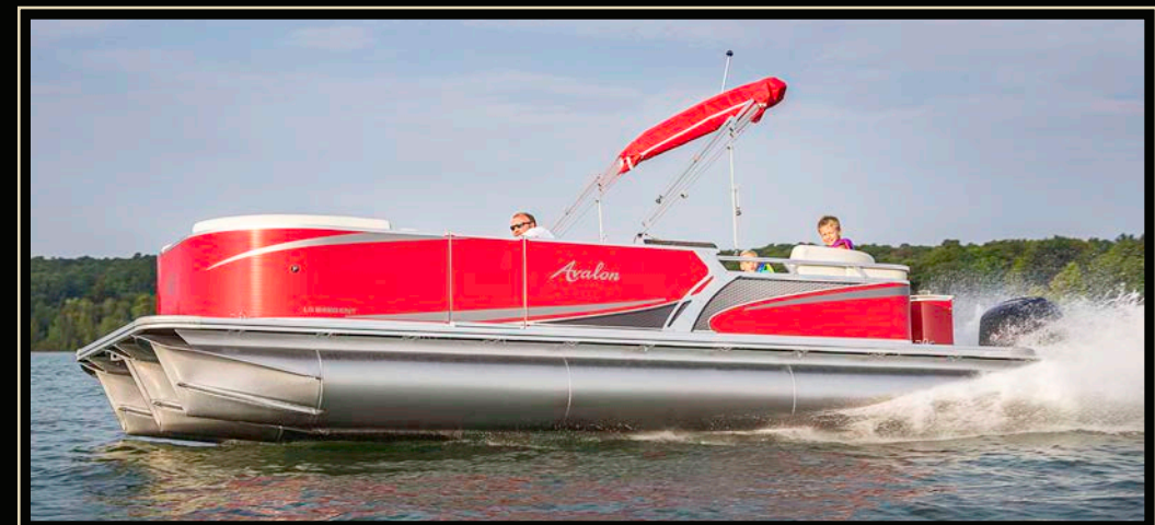
Turning package for Compact models – triple pontoons with internal fins for excellent lift and radical turns.
