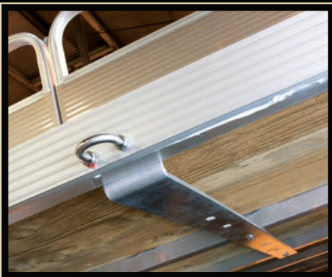
Strongest bow eye connected to 3 crossbeams
