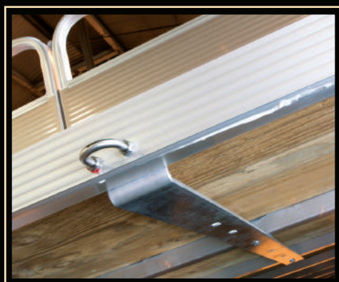
Strongest bow eye connected to 3 crossbeams
