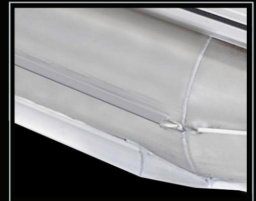
Exclusive side protector keel – protects pontoon from side impact at docks, provides a spray diversion, and makes pontoon structure stronger.
