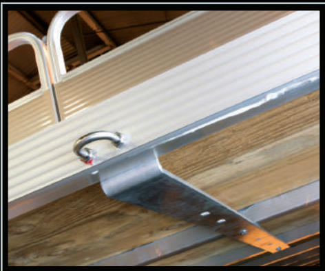
Strongest bow eye connected to 3 crossbeams
