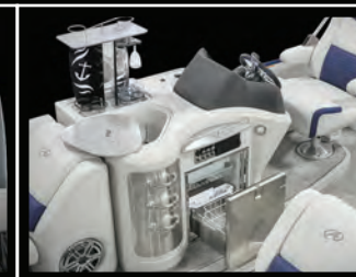
Admiral's Stand with Sink, Refrigerator, Electric Wine Rack and SST Drawers
