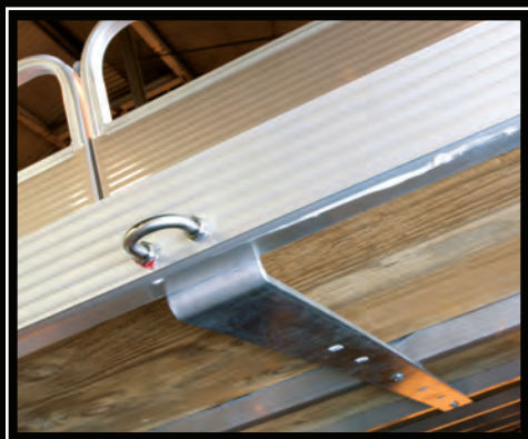
Strongest bow eye connected to 3 crossbeams
