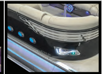
Built In LED Accent Docklights and External Lighted Air Vents
