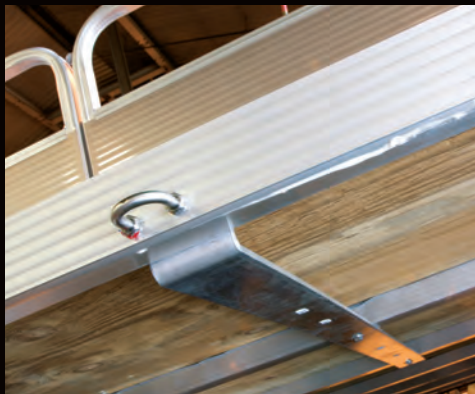
Strongest bow eye connected to 3 crossbeams
