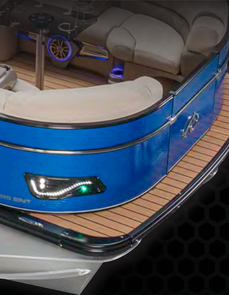
Docklights built into walls are protected from impact and are not a trip hazard! Nose cone tips covered by deck are less prone to damage and are less dangerous than exposed.
