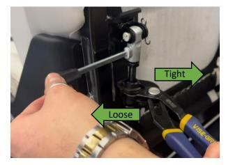
5. Apply blue thread locker on threads of the gas spring and tighten the nut against the release head while holding the gas spring in place with vice grips to prevent the lever from coming loose again.
