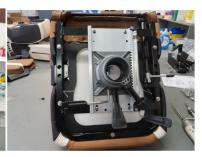
\*\*Notes: Gas spring on original frame can be salvaged if in working condition as a backup/replacement part for future use.
