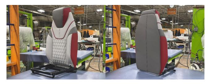
**5.** Verify the new frame has the gas spring installed as well as the Wieland Motion Badge shown below before continuing to the next steps:
