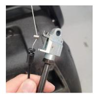
5. Flip the chair back over and locate the aluminum nut on the backside of the Push Button case. Using the channel-lock pliers, remove the nut from the case.
