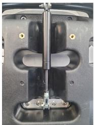
9. Clip the end of the cable assembly into the release head of the cylinder assembly. There should be a solid "Pop" into place.
