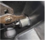
6. Once the nut is off the cable assembly, the assembly can be removed from the chair frame.
