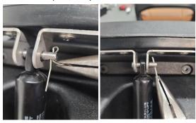
3. Remove the Pins and remove the cylinder from under the chair.
