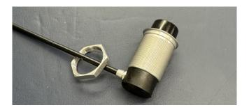
2. Insert the cable assembly into the hole in the chair. Run the nut over the cable on the inside of the chair and start threading it onto the aluminum push button case.
