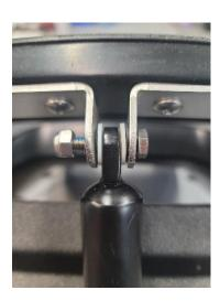
7. The release head end of the cylinder is attached the same way, just without the washers.
