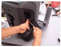
2. On the bottom of the chair, using the needle-nosed pliers, bend the clips back to be able to remove them from the pins, they will not be reused.
