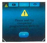
9. Once the update process has complete the screen will provide information to the user depicting so. It is then safe to turn the boat's battery switch off and then back on to reboot the Medallion Viper II module.
