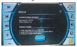
7. Press "Update". This will initiate update process and a screen prompt will present in the center of the 12" display. The screen prompt will provide the user update status. "Do not power off the unit or remove the USB stick during the update process"
